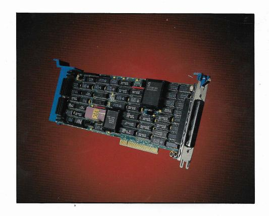
The 7-XP/2 is a convenient, simple way to run your DX10 applications on an IBM PS/2 or clone.
