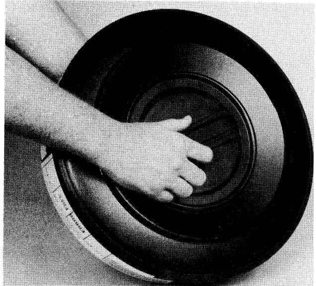
Removing the DS80/DS300 Disk Pack Lower Cover
